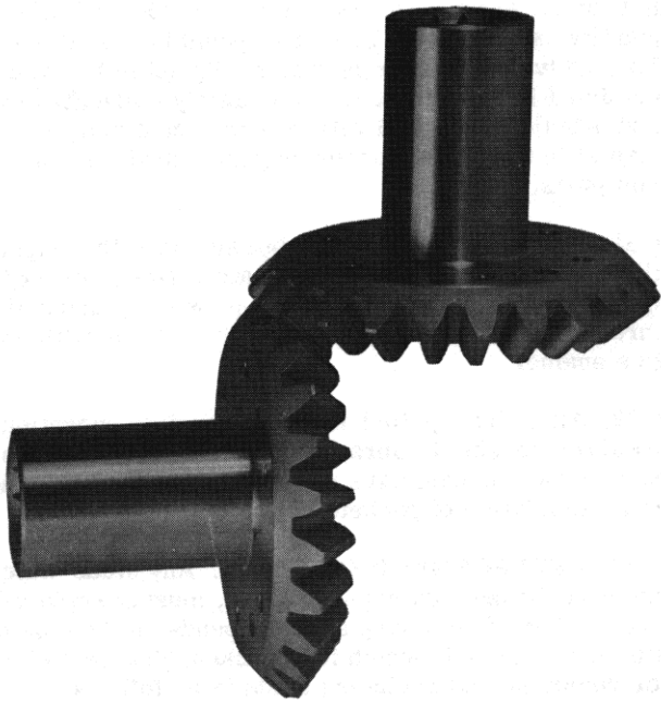
Figure 3-1. Bevel Gear - Showing Extreme Pitch Alignment
