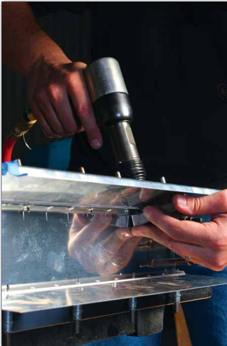
Solo riveting means holding the gun carefully in one hand and managing the bucking bar in the other. It's harder than it looks but gets easier with practice.
