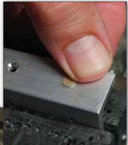
The problem when the countersink is too shallow (as shown by the right most rivet at left) is that the head isn't fully contacting the material and, therefore, the joint will not be full strength. Above: You can feel when the rivet “stands proud” of the material.
