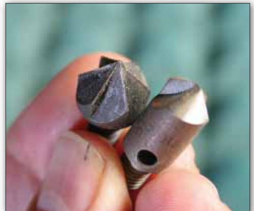
The deburring cutters come in a variety of sizes and countersink angles.
