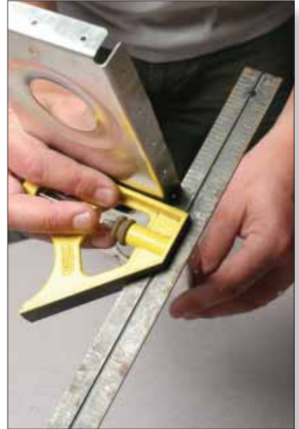
You can slide a square all along the flange to determine if it is perpendicular to the web of the rib or bulkhead. Be aware that some ribs may require something other than a 90° angle.
