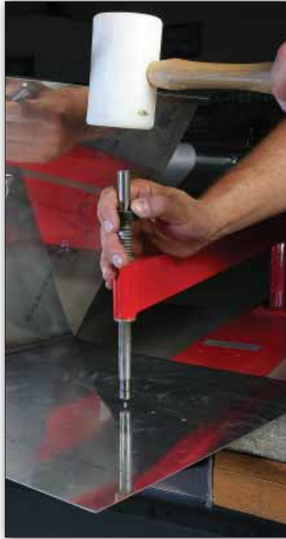
The C frame dimpler/riveter makes relatively quick work of the process. To use, carefully position the work over the dies (not shown here) and smack the head of the tool with a hammer.
