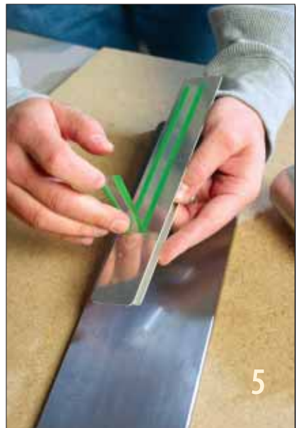
Work carefully while back riveting, as you do with other processes, and be sure that you steady the rivet gun with your free hand (4). When you're finished, simply peel the rivet tape from the part (5) and enjoy having that rare thing: a perfect part.
