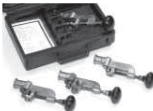
The Rivet Reader will give you a quick check of the proper set tail dimension. It should fit between the MIN and MAX lines.
