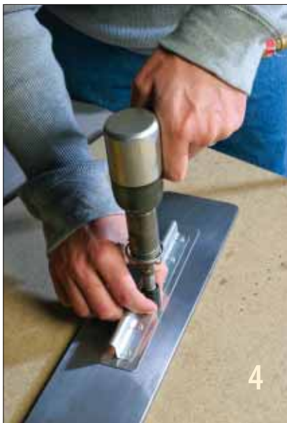
Work carefully while back riveting, as you do with other processes, and be sure that you steady the rivet gun with your free hand (4). When you're finished, simply peel the rivet tape from the part (5) and enjoy having that rare thing: a perfect part.
