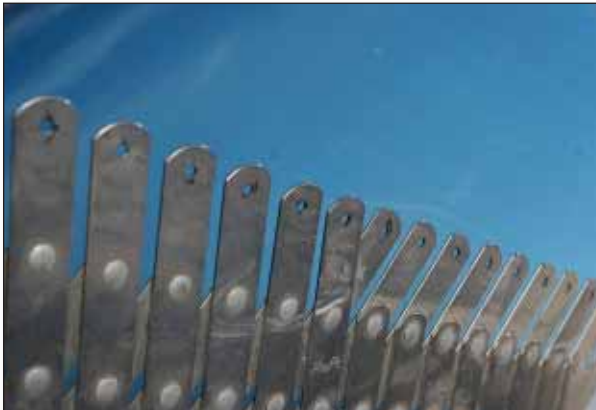
This is not a set of conjoined feeler gauges. A rivet spacer like this will help you distribute a line of rivets evenly—and, most importantly, help your work look nice.
