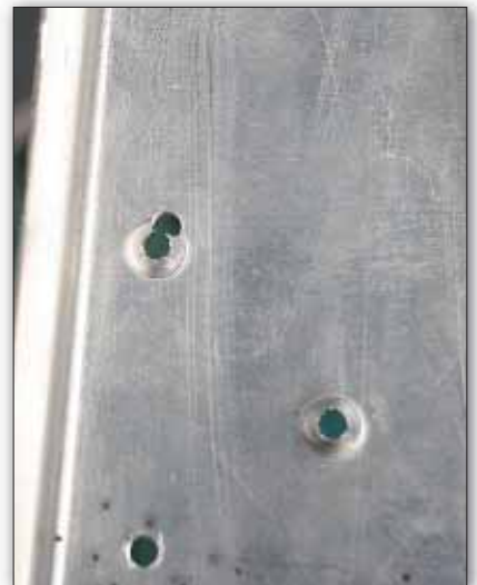
It's the big whoops: You've pulled the trigger and the male die slipped out of the hole. You were either slightly off (top left) or way off (right). Believe it or not, there's a way to fix this. (See text.)
