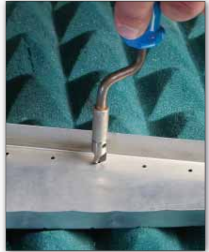
A "speed deburr" tool uses a simple fluted bit on an offset handle. One turn and you're done.
