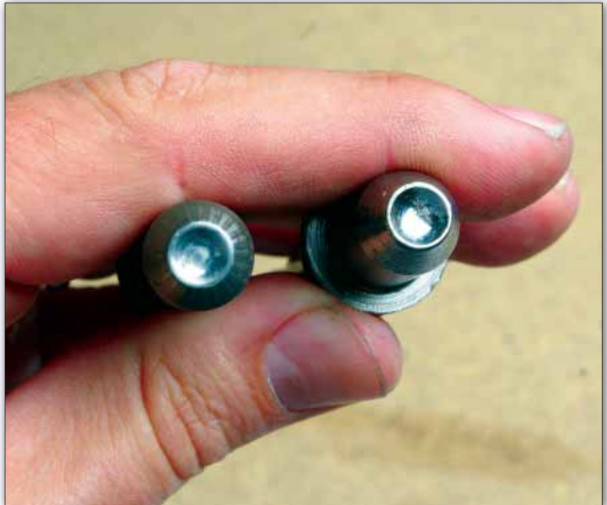
Rivet sets for driving protruding-head rivets have a specially designed recess intended to press evenly on the manufactured head.
