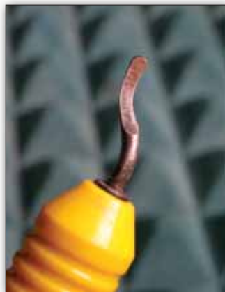
For deburring large pieces, use this hook-shaped tool. As with all deburring, a little bit will do the job. Don't take a lot of material off.
