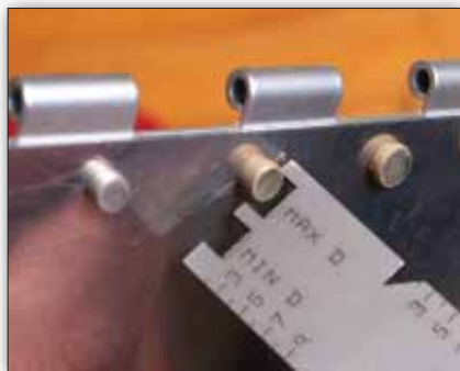
The Rivet Reader will give you a quick check of the proper set tail dimension. It should fit between the MIN and MAX lines.
