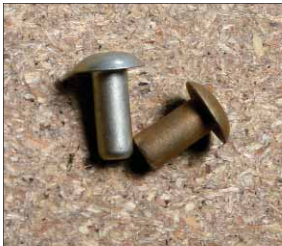
And the after effects: The rivet on the right has been carefully squeezed, like a tiny marshmallow man. Use care and discard any homemade oops rivets that are wavy or tipped.
