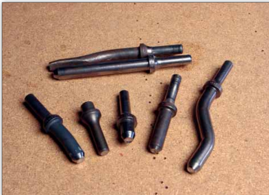
You will find a need for several rivet sets, including straight sets, angled sets and offset versions with a built-in S curve.
