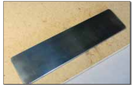
The back riveting plate is simply a smooth, heavy slab of steel that will be your stationary bucking bar.
