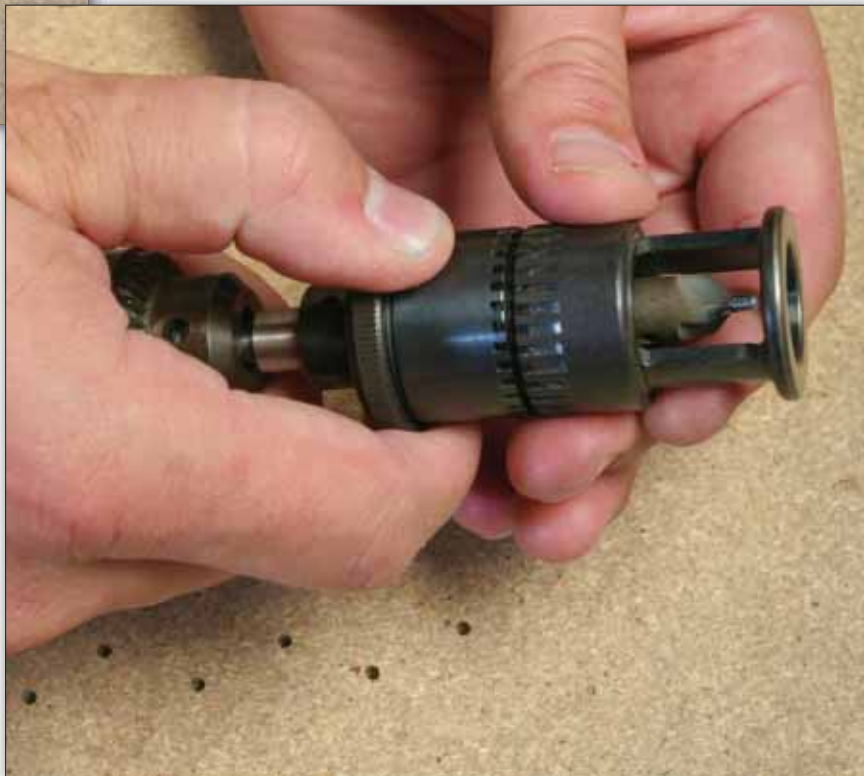
These serrations on the barrel of the microstop set the depth of the cut to a very fine degree. Once set, the tool holds its calibration well, allowing repetitive countersinking with great accuracy.
