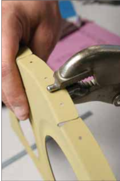
Fluting pliers clamp down on the flange and form little notches to straighten the part. Make sure you've got the tool oriented correctly—the notches should be formed away from the adjacent part.
