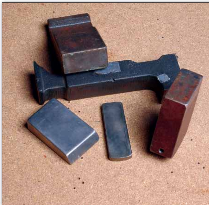
Bucking bars, you'll have 'em by the dozen. Differing shapes and sizes will help you buck rivets in even the most cramped quarters.
