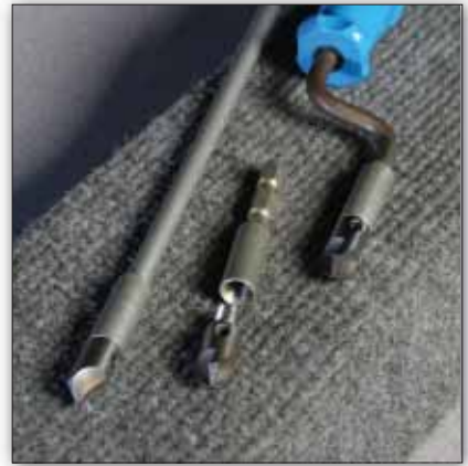
The deburring sets come in a variety of configurations. You've got your extension handle (left), drill chuck version (center) and basic speed handle (right).
