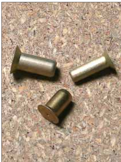
Premade oops rivets have the standard head size but a larger shank—the rivet facing down is one of this clan.
