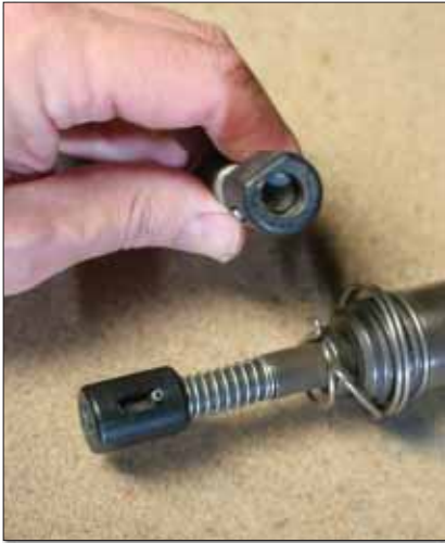
A special back riveting set keeps the gun centered on the bucktails and helps you create perfectly set rivets.
