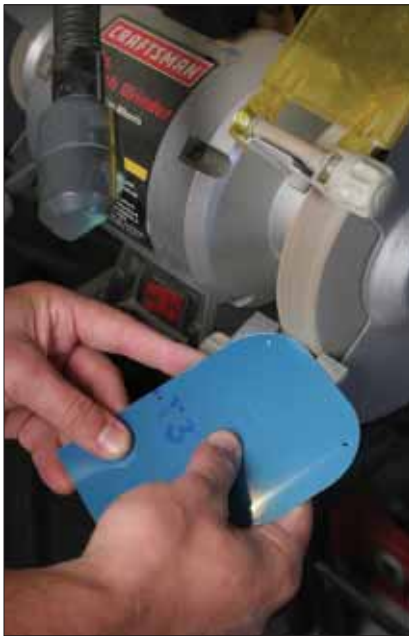
Commonly referred to as the “Scotch Brite wheel,” the 3M Cut & Polish wheel can be mounted on a bench grinder or a drill press.
