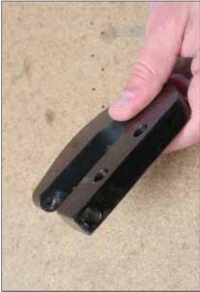
The yoke: It attaches to the squeezer body with two bolts or pins, has a hole in the bottom for the plunger, and typically has a hole in the top for a set or dimple die.
