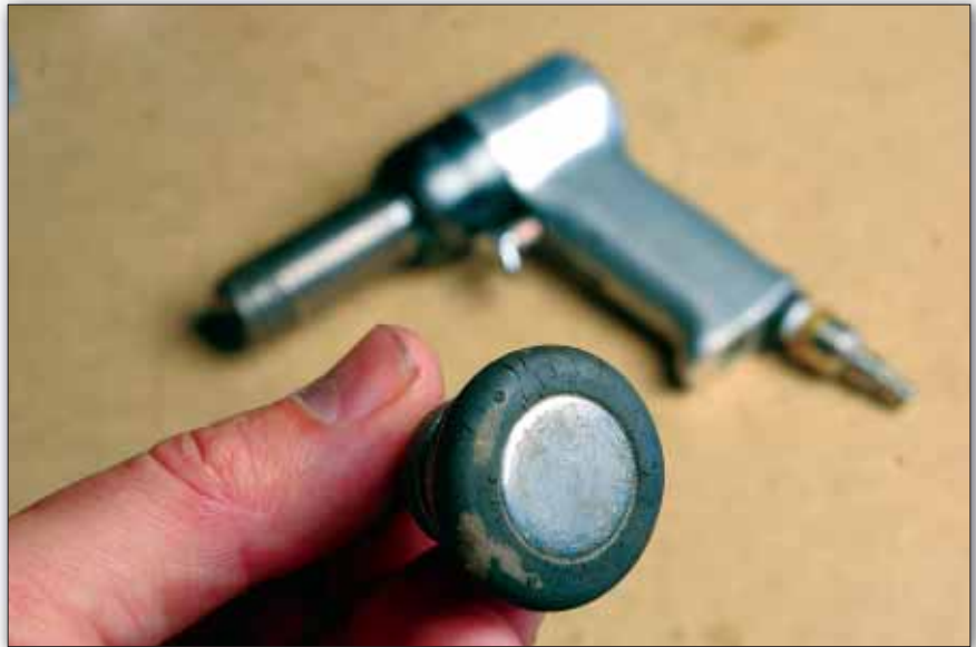
A flush rivet set uses a flat-faced shoe in the rivet gun to apply impacts to the manufactured head of flush rivets. The rubber surround helps prevent marring the surface.
