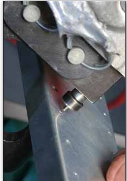
Used in a pneumatic squeezer, the dimpling die makes quick work of thin material. Just be careful of where you put the tool, and know before you pull the trigger which side you're supposed to be dimpling!
