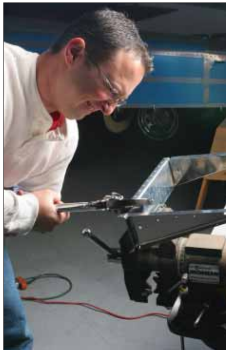
Using a hand squeezer is satisfying work, but it's tiring at best. If you're on a tight budget, get used to this pain. Otherwise, the pneumatic squeezer is worth its weight in gold.
