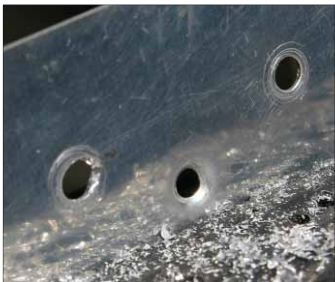
Bad, good, bad: If you continue to drill through the material to remove the rivet, you will almost certainly enlarge or elongate the hole. Your best choice now is to drive an oops rivet.
