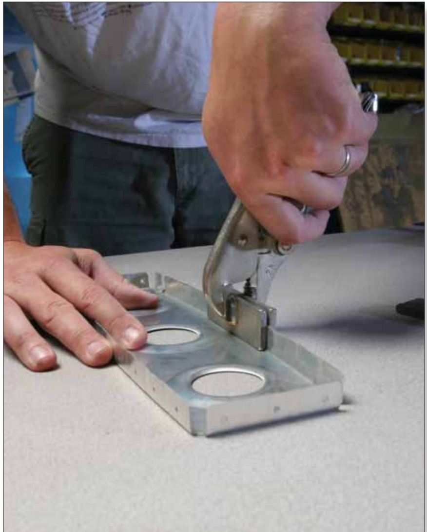
A hand seamer has more uses than simply bending metal. It can also be used to change the angle of flanges, or to squeeze out flutes if you overdo it when fluting.
