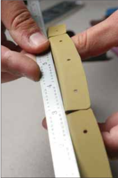
Flanges often need a fair amount of straightening. Use a straightedge to gauge how much curvature needs to be taken out by the fluting process. Go slow, it's an iterative process that requires finesse.
