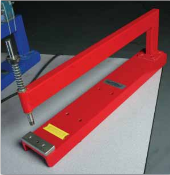
The C frame dimpler/riveter makes relatively quick work of the process. To use, carefully position the work over the dies (not shown here) and smack the head of the tool with a hammer.
