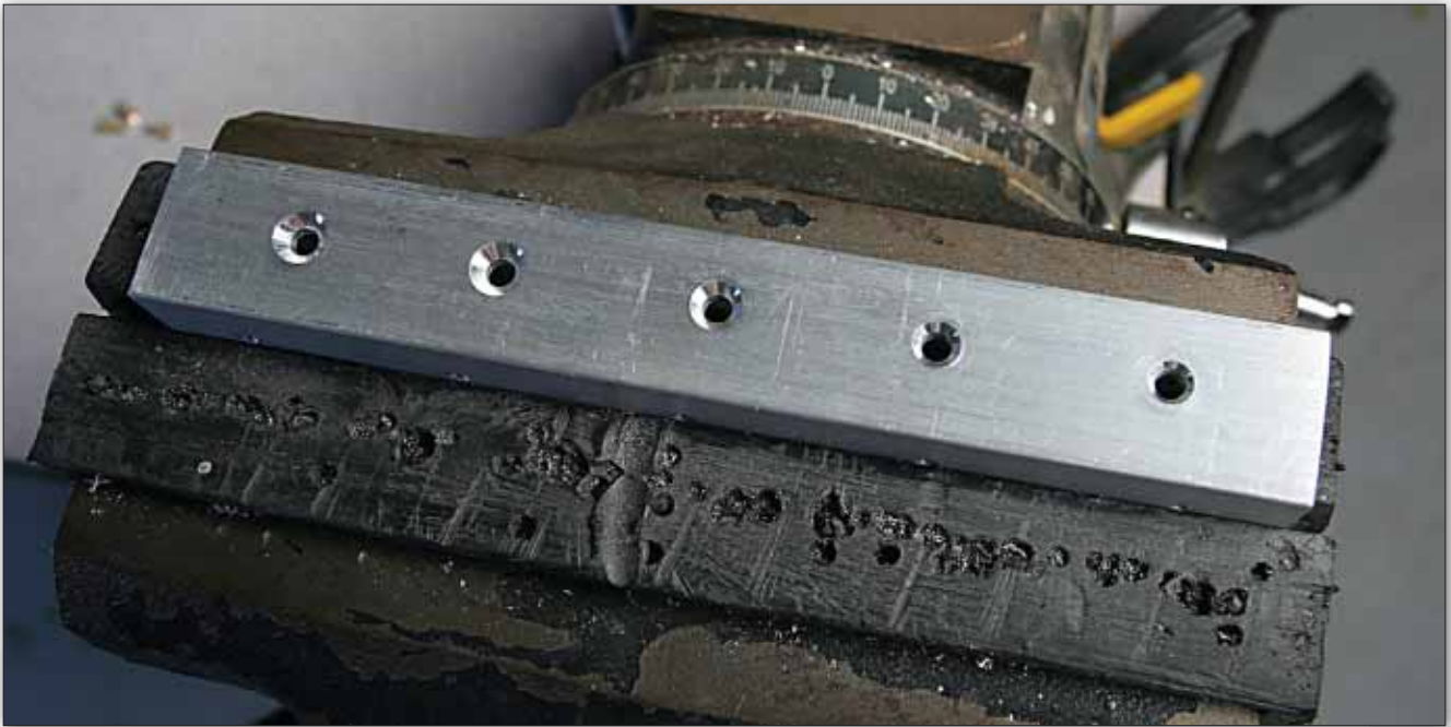
The five stages of countersinking, from left to right: Too deep with the pilot going off center and causing chatter; still too deep but at least it's smooth; just right; too shallow; and way, way too shallow. Trial and error, together with careful setting of your microstop bit, will help.
