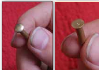
The AN470 round-head rivet (left) and AN426 countersunk rivet are staples—pardon the pun—of modern metal aircraft.
