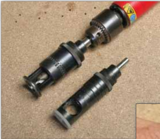
The heavy-duty microstop is in the drill; the standard version below. Buy the best.
