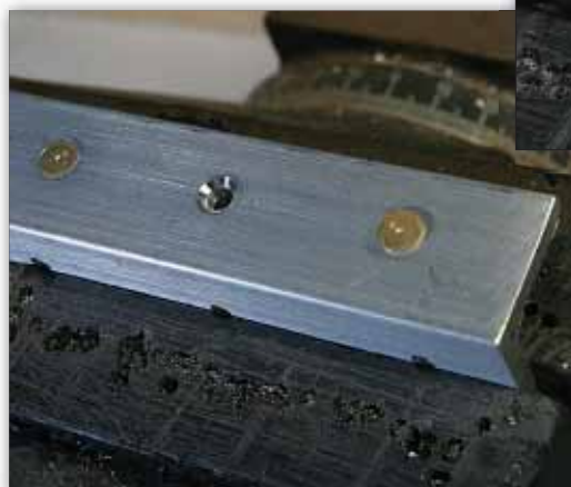
The problem when the countersink is too shallow (as shown by the right most rivet at left) is that the head isn't fully contacting the material and, therefore, the joint will not be full strength. Above: You can feel when the rivet “stands proud” of the material.
