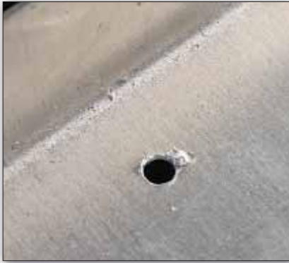
The burr. No matter how sharp your drill bits, the act of drilling will leave chips and flakes behind. Deburring takes this junk off. Simple as that.
