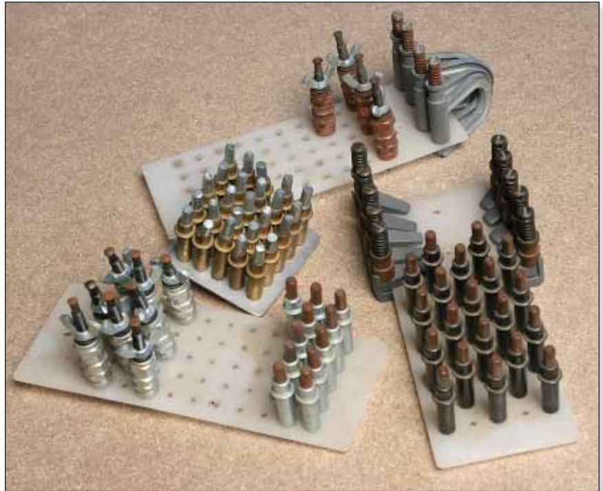
Clecos come in a wide variety of shapes and sizes, and include special C-shaped versions to hold sheets of metal by the edges.
