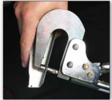
Hand squeezers can do more than just squeeze rivets. They're great at dimpling holes in flanges.
