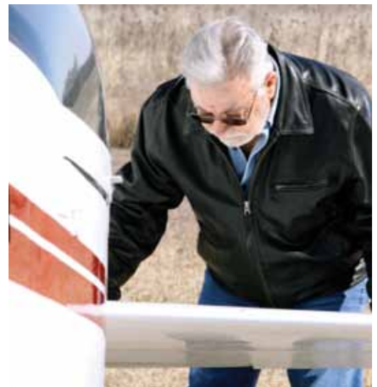
DAR Mel Asberry checks the manual trim on his airplane. Manual flaps also serve his purposes and keep the systems simple.
