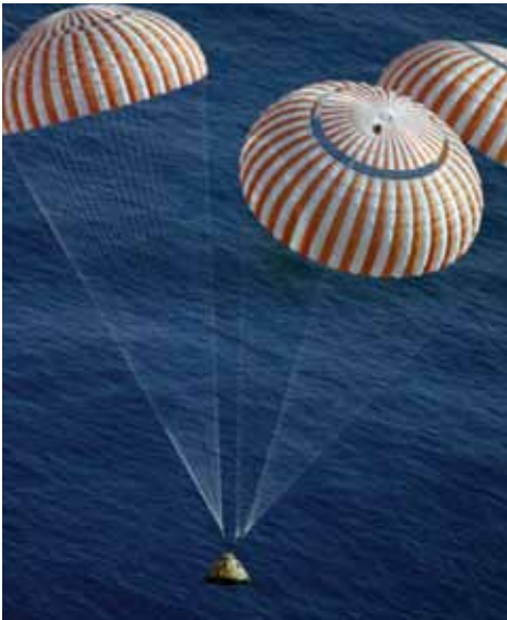
The Apollo spacecraft returned to earth via parachutes, and they were tested with boilerplate mockups many times before humans rode them home from space.
