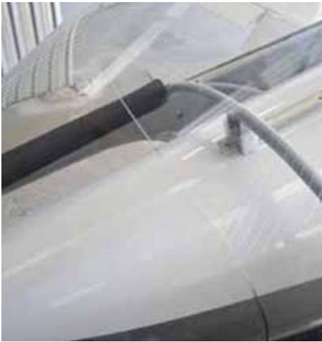
All it takes to cause a crack in acrylic is a single rivet hole with a burr or microcrack. Take the time to polish edges and holes correctly.
