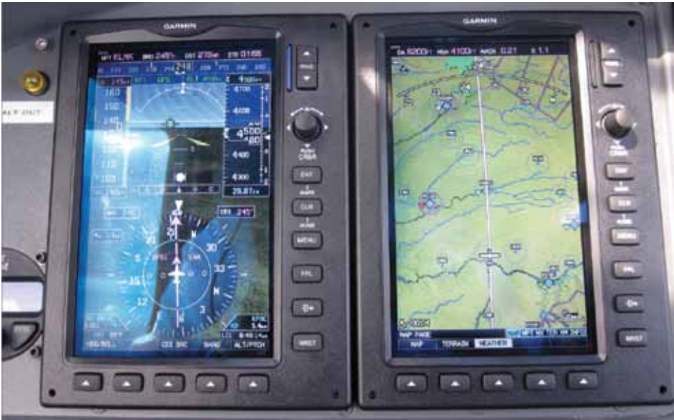
Having two EFIS screens provides a backup in case one fails—as long as they aren't both rendered inoperative due to a common power loss. How you power expensive equipment is as important as having the equipment.
