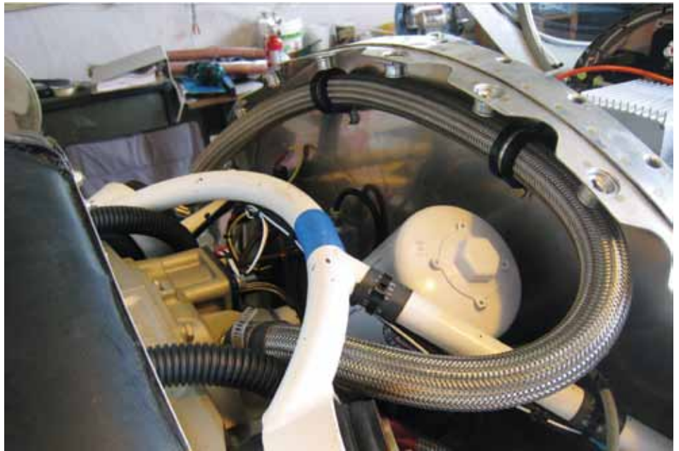
Details in the engine compartment mean padding the mount tubes with rubber or silicone tape if you need to attach a wire tie.
